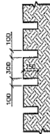
STAIR HOLES TYPICAL DETAILS SCALE 1:50 (SEE NOTE 13)
